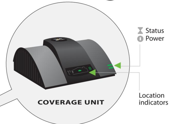
Set Coverage Unit near the middle of your home and plug it into the nearest outlet. Wait until the status light stops flashing. **You should see this on the Coverage Unit indicator panel.**
